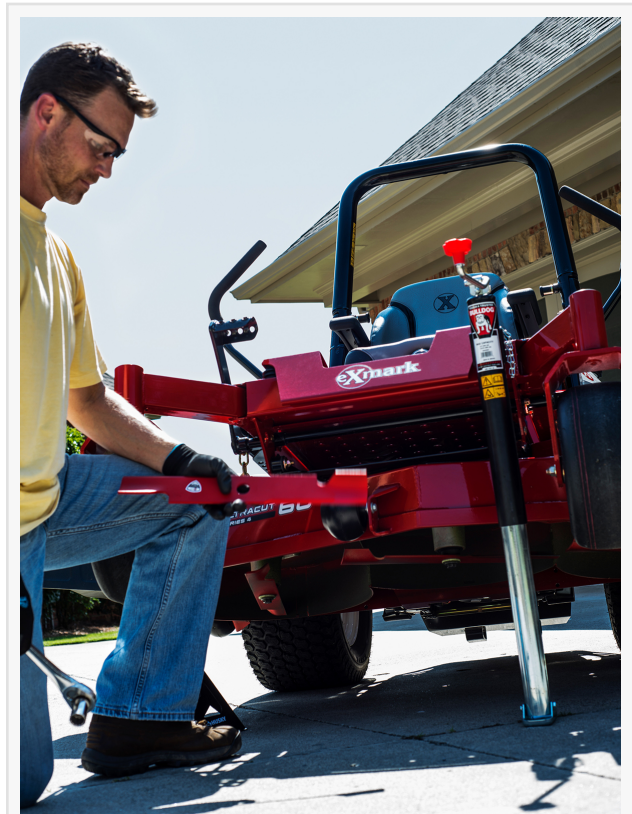
Sharp mower blades help the mower cut grass blades cleanly, improving finished cut quality and turf health.
