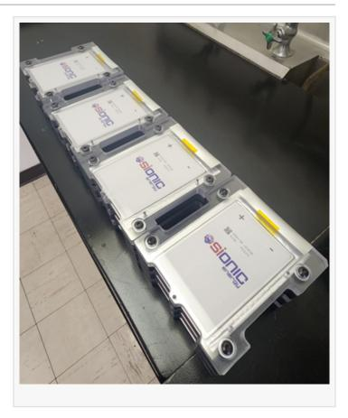
As demand for high-performance, sustainable battery solutions continues to grow, Sionic's technology offers a game-changing advantage — boosting energy density by up to 42% over conventional lithium-ion batteries while cutting charge times to as little as 10 minutes. By leveraging a proprietary silicon anode and advanced electrolyte system, the platform enhances battery efficiency without requiring costly manufacturing overhauls, ensuring a scalable, cost-effective path to commercialization.
