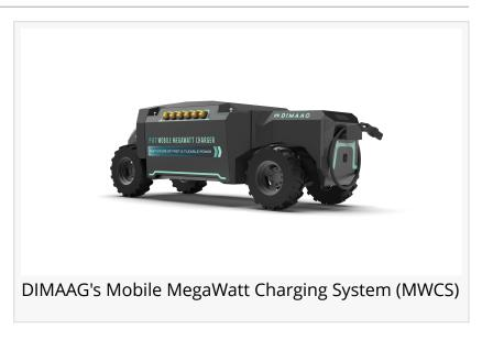
off-road applications, the MWCS enables charging at point of use, thereby significantly reducing downtime associated with trips to fixed charging stations.
