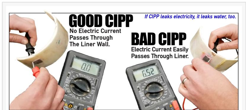
Low voltage conductivity allows utilities to automatically identify location and severity of defects in Cured-In-Place Pipe (CIPP) and other trenchless rehabilitation.
