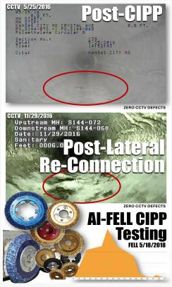
Another common reason for CIPP to leak more after rehabilitation is damage caused by Post-CIPP CCTV inspection and/or lateral reinstatement equipment.
