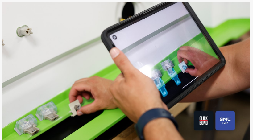
Mixed reality is used to show exactly where a Click Bond part should be placed, improving precision
