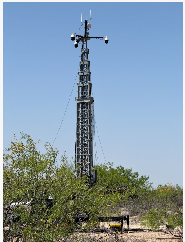
Skylark Labs Scout Mk II tower with Pierce Aerospace's YR1 Remote ID Sensor and visual sensors was deployed to Mexico. The tower stands at 100 feet and is actively detecting and tracking UAS along the Mexico-US border.
