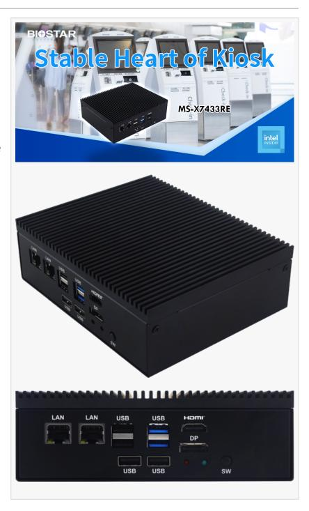
includes a SATA III port alongside an M.2 Key-M slot, enabling both traditional and high-speed NVMe storage. A Mini-PCIe slot and M.2 Key-B interface with support for 4G/5G modules make it
