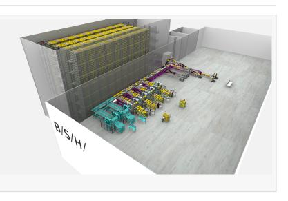
warehouse that will supply production with components reliably and quickly. More than 50 shuttle robots will ensure that the required components are supplied to the assembly workstations at just the right moment.
