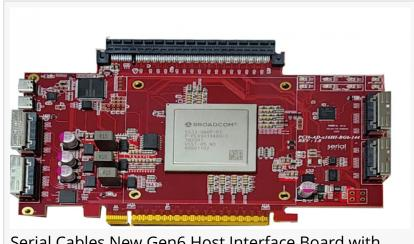
Serial Cables New Gen6 Host Interface Board with Broadcom PEX-90144-A0-1 Atlas III Switch Chip
