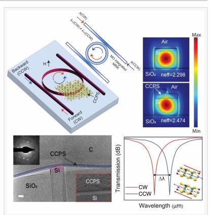
a, Schematic of the CCPS/Si microring resonator under an applied magnetic field, showing CW and CCW light propagation differences. b, Electric field intensity profiles for TE modes at 1550 nm for bare and CCPS-integrated waveguides. c, TEM crosssection o
