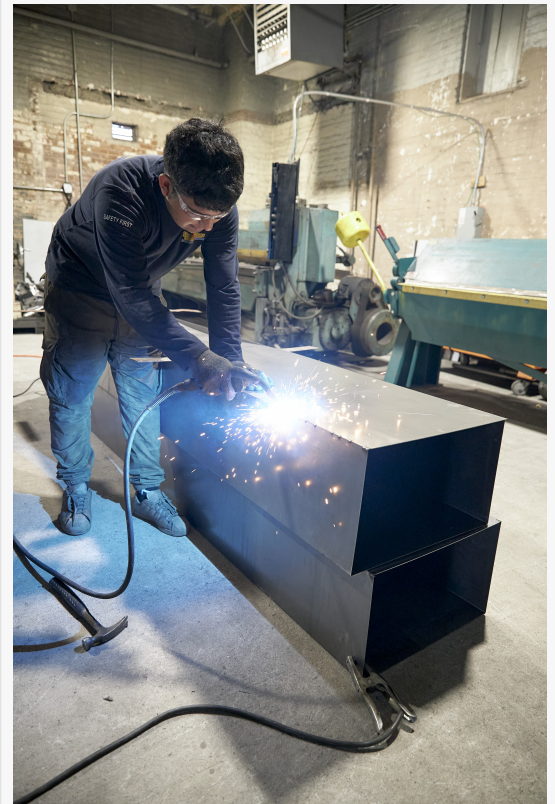
Done Right fabrication team welding a NFPA 96 code-compliant exhaust systems.
