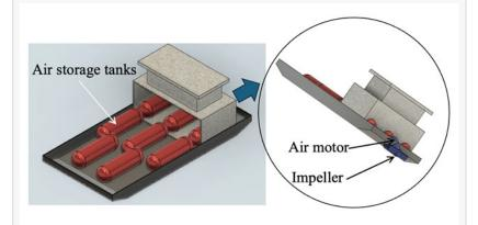
The research findings are based on experimental results and realistic calculations using polytropic relations to realistically calculate the behavior of the air from being pressurized in the tank, flowing into the air motor that is used to rotate the prop
