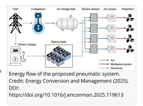
"Replacing these engines with pneumatic ones is a cleaner and more effective option as these engines can also be incorporated into the ferry body to store air either within the structure of the boat or on auxiliary tanks, which will enhance buoyancy," said Abdul Hai Alami, the lead author.
