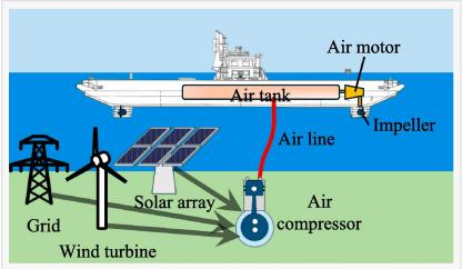
Schematic of the proposed pneumatic propulsion with multi-option for connectivity, be it grid and/or renewable energy connectivity. Credit: Energy Conversion and Management (2025). DOI: https://doi.org/10.1016/j.enconman.2025.119613
