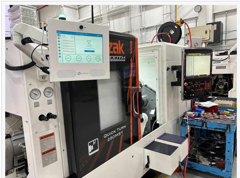
Harmoni device connecting the machining center, operator, and ERP together
