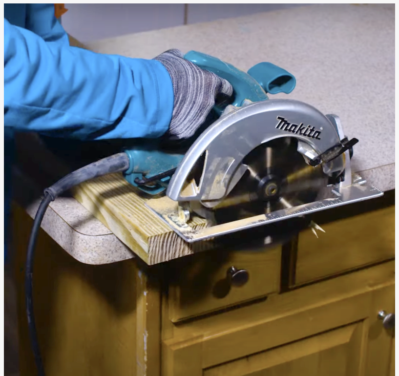
Prior to assembly, a circular saw is used to cut all boards to length.
