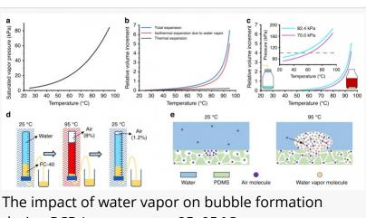
The impact of water vapor on bubble formation during PCR (temperature: 25–95 °C, pressure: 101.325 kPa).
