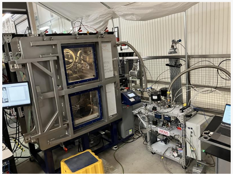
LUNAR's LR-1 MRE reactor operating in NASA's Kennedy Space Center Assist Chamber
