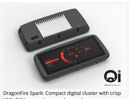
DragonFire Spark: Compact digital cluster with crisp HMI, CAN connections, and rugged housing—optimized for fleet integration.
