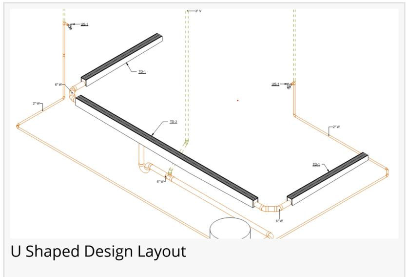
The system features a u-shaped 6 inch wide pre-sloped trench drain equipped with stainless steel grates and high-density polyethylene (HDPE) channels. This combination offers chemical resistance, corrosion protection, and long-term durability—making it particularly well-suited for the harsh environments typically found in wastewater treatment operations. The use of HDPE channels ensures lightweight handling and ease of installation, while the stainless steel grates provide sustained use.
