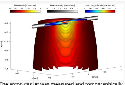
The argon gas jet was measured and tomographically reconstructed with a back pressure of 7.5 bar and a laser intensity of 0.5 mJ. The maximum ions charge density is , and the maximum gas density is . Gas jet is visualized as cut-outs within isosurfaces
