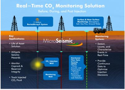
Real-Time Class IV Well Carbon Monitoring System - Before, During, and After Injection
