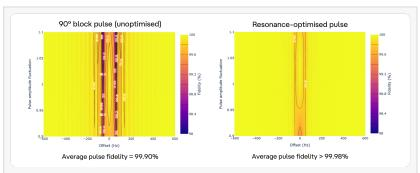
Resonance-optimised pulses (average fidelity > 99.98%) are more robust to B0 and B1 fluctuations than conventional block pulses (average fidelity = 99.90%).
