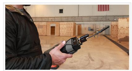
WhiteFox Defense's Scorpion 3 handheld counterdrone system provides rapid, real-time drone detection and tracking capabilities for tactical teams operating in dynamic environments.
