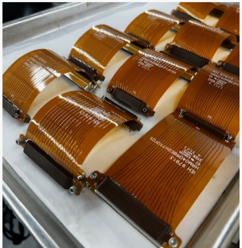
IEH engineering work with clients on the design and layout of flex assemblies, sources them and terminates them to IEH connectors
