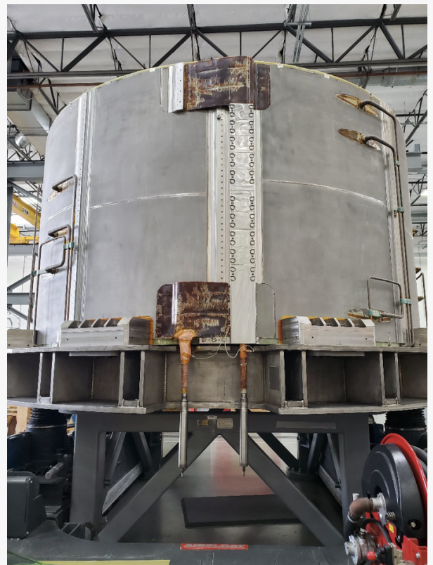
The sixth module of the Central Solenoid, completed at General Atomics in April 2025. When combined with the five other completed modules, the Central Solenoid will form the center of the ITER tokamak and the pulsed magnet system.
