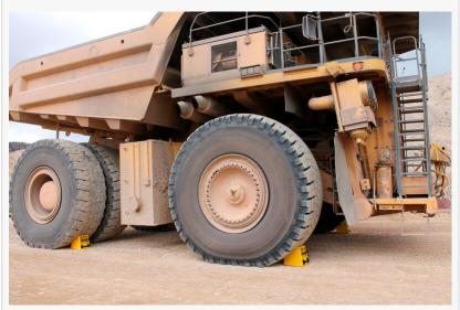
Manufactured in the USA, Checkers new ultra-class wheel chock meets MSHA specifications and is constructed from weather-resistant HDPE, which also makes it resistant to oils, fuels, and solvents typically found in mining environments.
