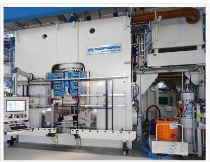
The fully automated production of copper fittings on the Graebener® fitting press enables very short cycle times
