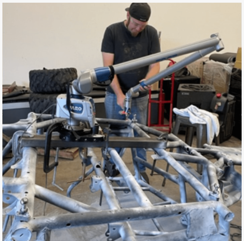
ScanToCad add-ins Industry 4.0 supports Portable CMMs for closed loop 3d probing and scanning direct in CAD
