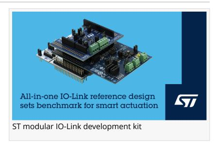
By including the actuator hardware, ST's <u>P-NUCLEO-IOD5A1</u> kit goes further to help users leverage IO-Link's powerful bidirectional point-to-point connectivity in all types of device nodes. Widely used in industrial-automation projects, the protocol enables rich interactions with sensors and actuators, including device configuration and diagnostic reporting as well as basic input/output data.
