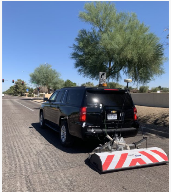
The high-speed 3D GPR array can capture accurate data at up to 80 mph
