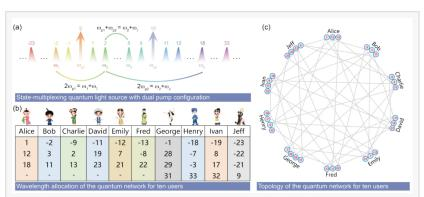
a, State-multiplexing quantum light source with dual pump configuration. b, Wavelength allocation of the quantum network for ten users. c, Topology of the quantum network for ten users.
