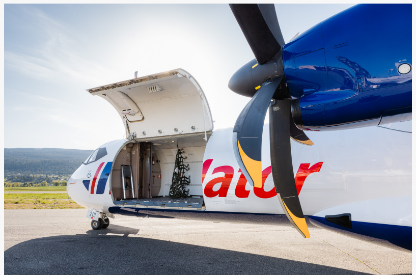
The ATR 72-500F was previously converted from a passenger to cargo aircraft by KF's in house experts.
