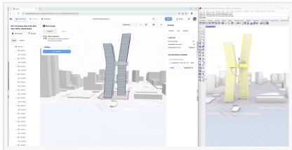
With Skema's integration with Rhino, architects and designers are now able to evolve Rhino designs into highly-constructable and trusted BIM models - without scripting, manual remodeling, or any loss of design intent.
