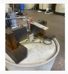
components and features a stable base, upright legs, and a top plate with a notch and locking mechanism to hold hoses securely in place.
