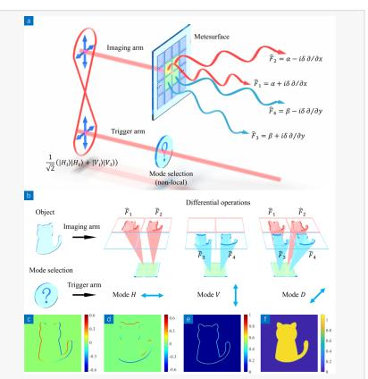
Phase reconstruction via metasurface-integrated quantum analog operation.
