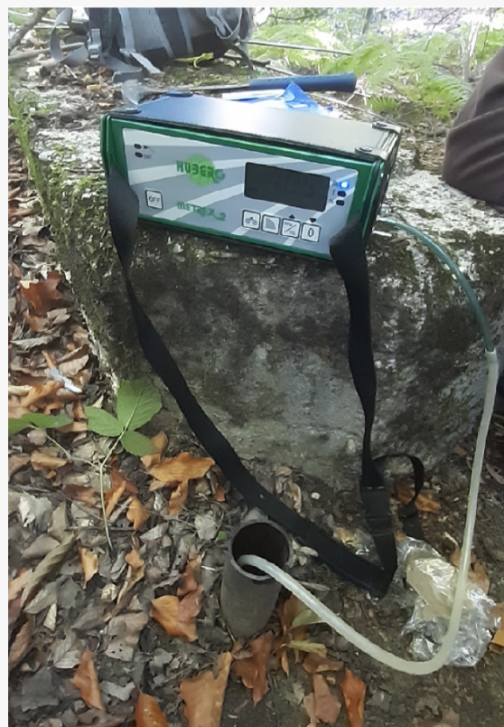
Measurement of Hidrogen by semiconductor sensor in Baia Nouă
