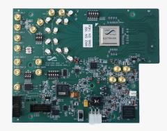
64GSPS 36GHz RF-Sampling Electra-M MX2 Evaluation Board
