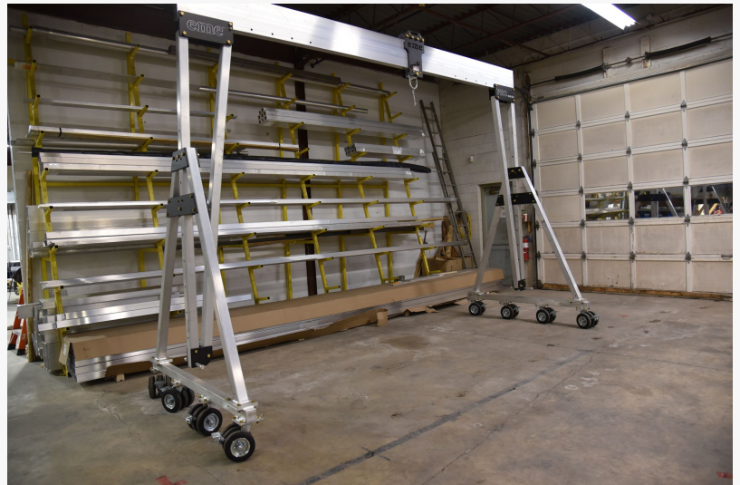
eme 6600R gantry crane shown with new 3 tonne-rated pneumatic casters, designed for full mobility under load.
