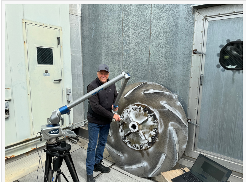
Reverse Engineering direct to Inventor with 7 axis PCMM - No Drawing exist for manufacturing
