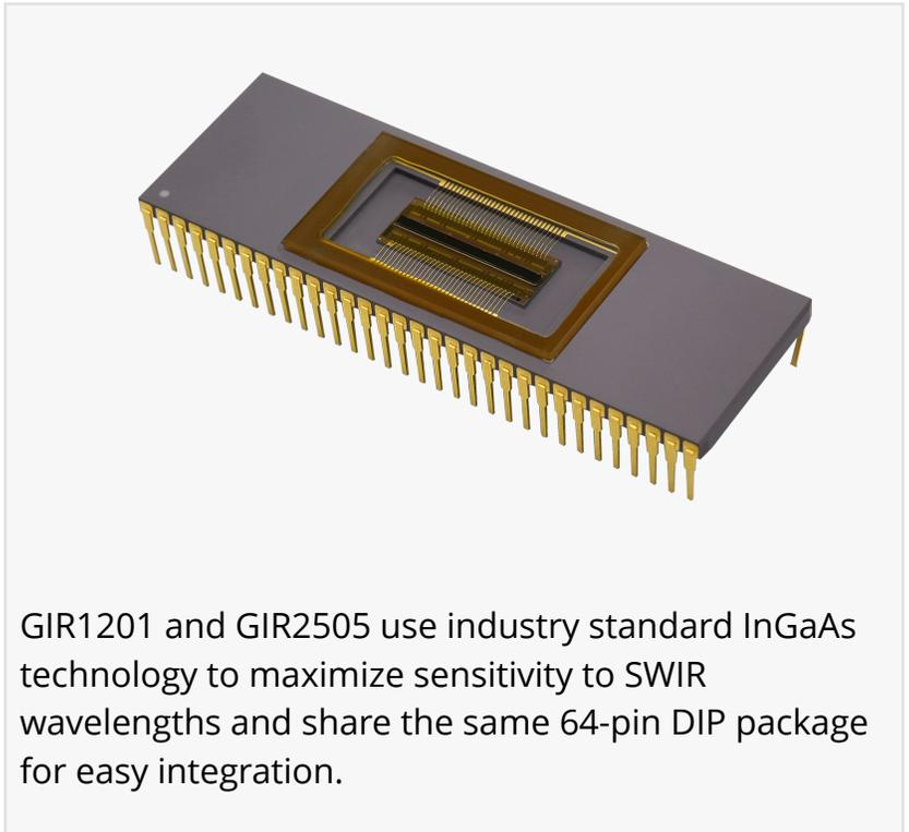
GIR1201 and GIR2505 use industry standard InGaAs technology to maximize sensitivity to SWIR wavelengths and share the same 64-pin DIP package for easy integration.
