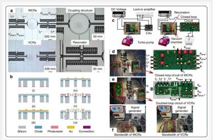
a Images of the coupled resonators. b Fabrication process for the coupled resonators. c Schematic of open-loop and closed-loop test. d Closed-loop test of WCRs. e Closed-loop test of VCRs. f Bandwidth test of WCRs and VCRs.
