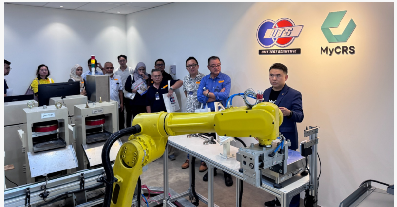
MyCRS x UTS Autonomous Concrete Testing System
