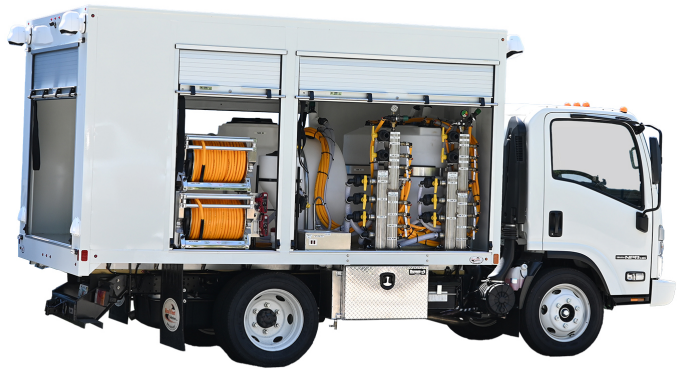
Side view of Real Fleet Solutions' Tree Spraying Truck with compartment open, revealing integrated equipment tanks, hose reels, and secure storage layout.
