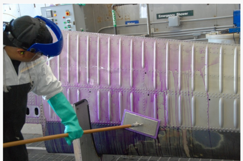
Application of CHEMEON eTCP to a UH-60 Stabilator at CCAD
