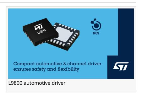
The L9800 outputs can drive resistive, capacitive, or inductive loads like relays, solenoids, and LEDs. With continuous real-time diagnostics and open-circuit, short-circuit, overcurrent, and overtemperature protection per channel, the L9800 enhances vehicle reliability and eases system-level ISO 26262 certification up to ASIL-B. The diagnostic signals are available at the L9800's SPI port, which also provides access to the driver's internal configuration registers for device set-up.
