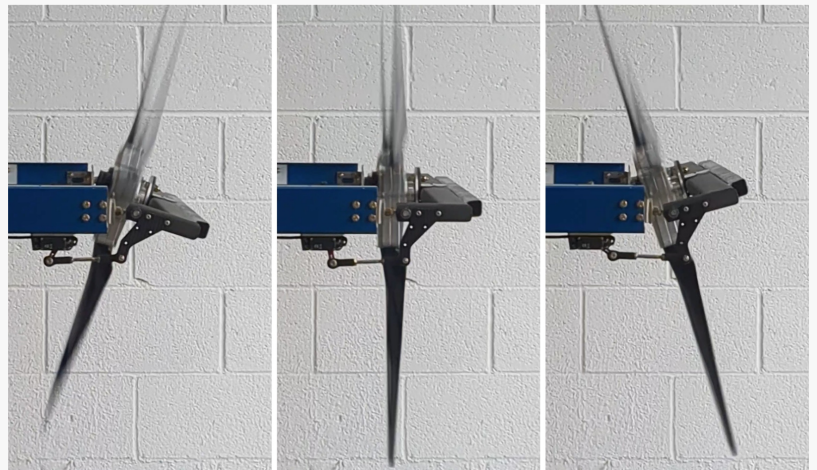
A rapid sequence of images showing the Thrust Vectoring Evaluation Kit propulsor being put through its paces on a test bench
