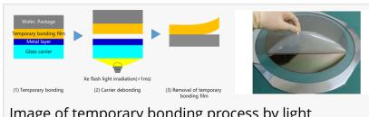
Image of temporary bonding process by light irradiation and easy removal of temporary bonding film by peeling off
