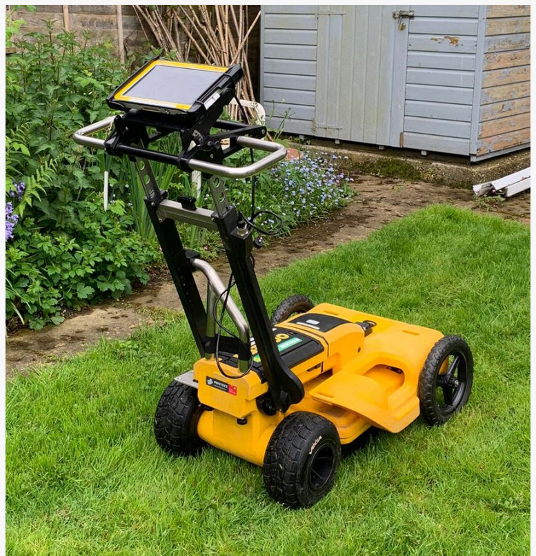
GPR Survey DS2000
