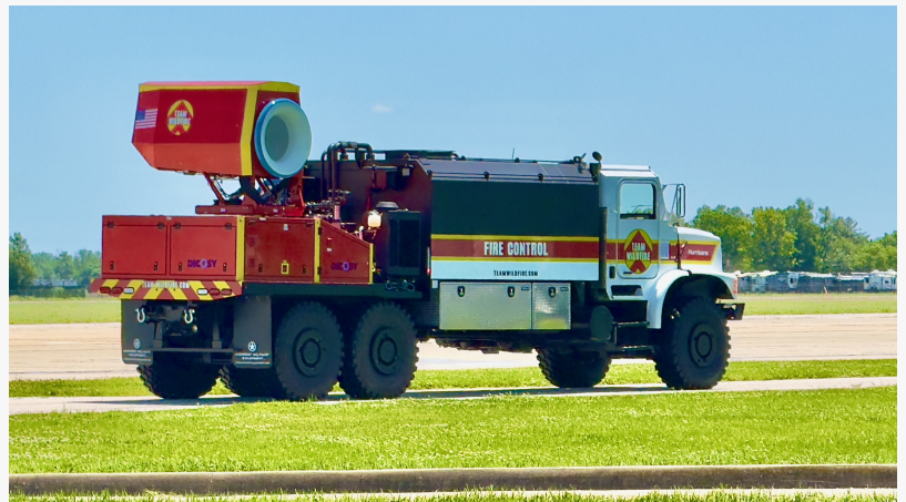
Team Wildfire's Hurricane uses a jet engine to blow back wildfires.
