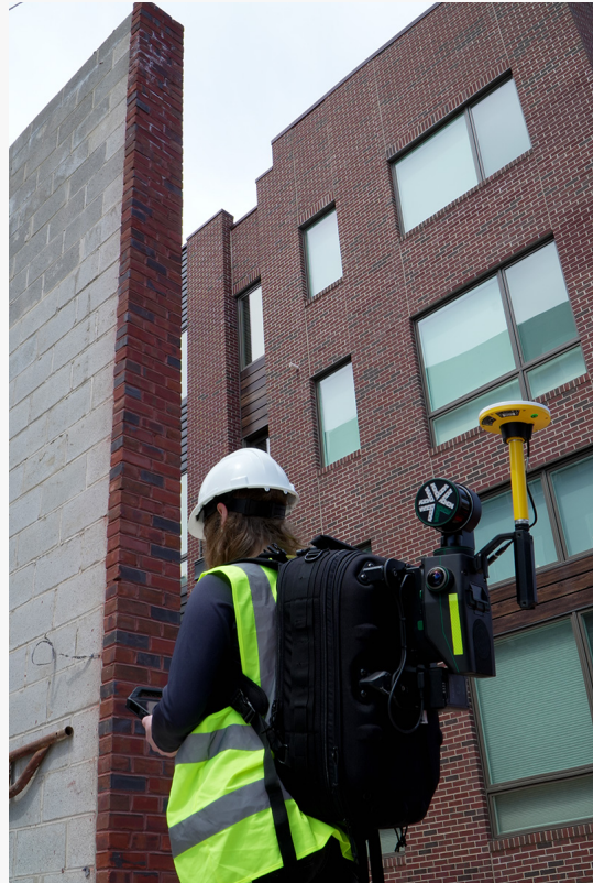
Trimble DA2 GNSS Mounted on Exyn Nexys at a Construction Site
